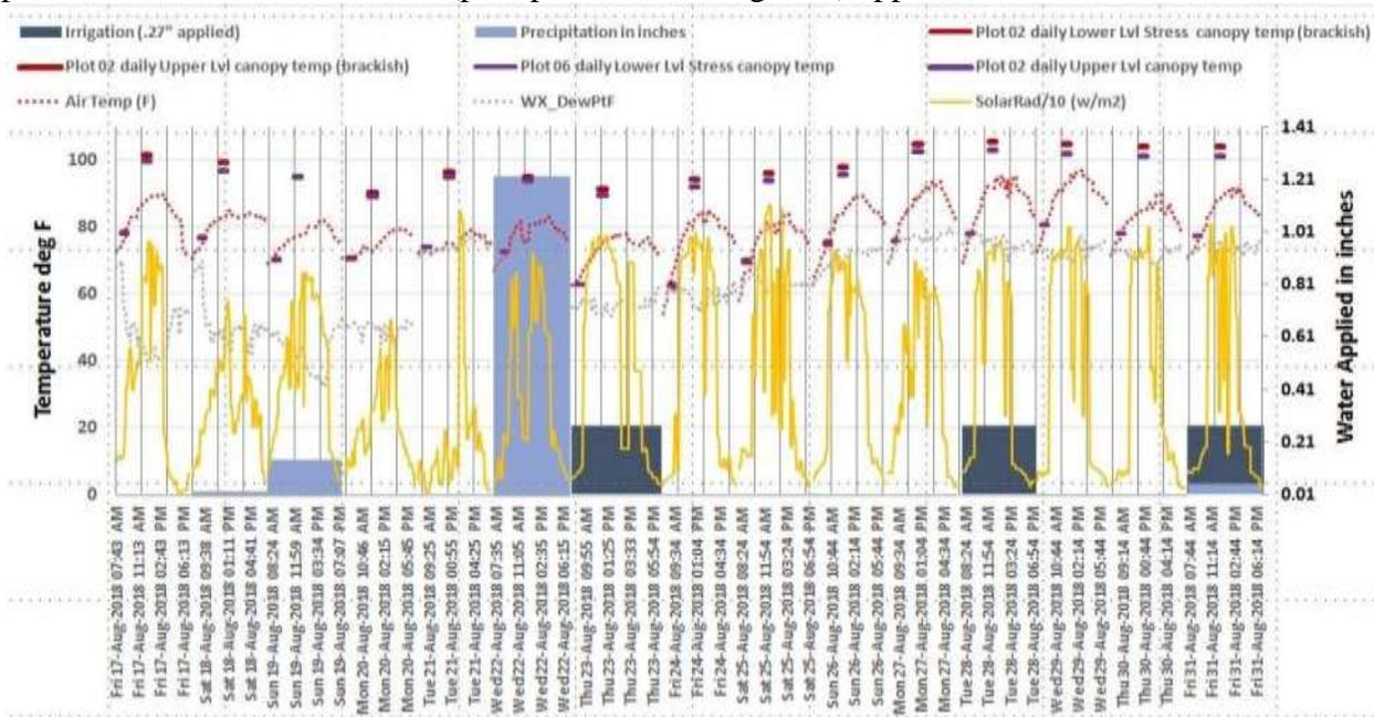
*Figure 10. Upper and Lower Stress Temperatures, Canopy Temperature and Water*
